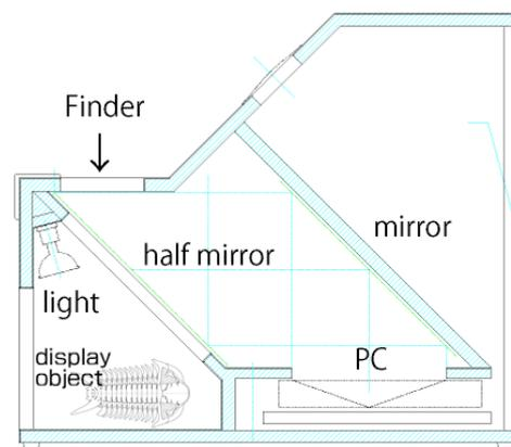
Fig. 3 Display box structure
